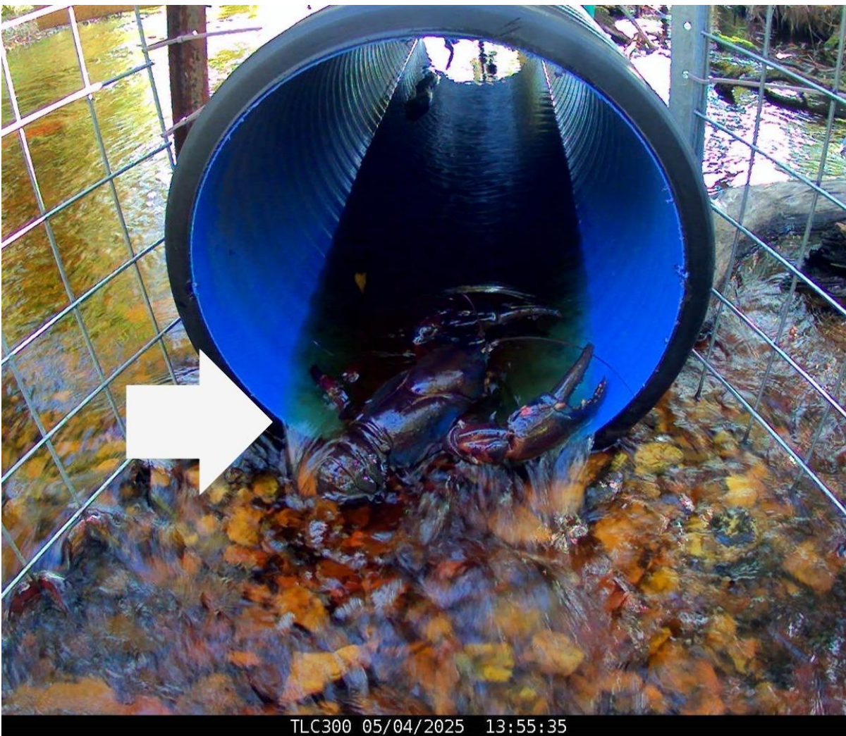
Picture 5. Placed GFC Unable to Gain Traction on Bare Culvert Base when Heading Upstream:
